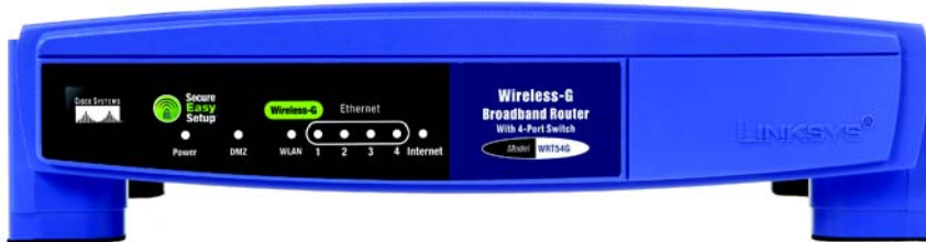
Figure 3-2: The Router's Front Panel
